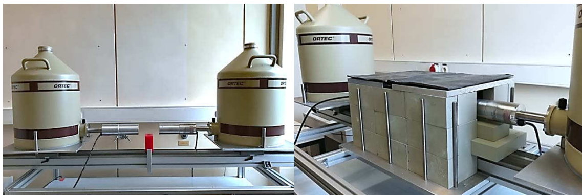
Fig. 1. Left: 2 HPGe detectors with a relative efficiency of 25% (left detector) and 22% (right detector) positioned on a slide guide. Right: Final gamma detector setup including lead shielding.
