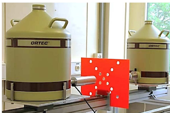
Fig. 3. HPGe detector setup including sample holder (red) for validation measurements with point sources at different angles from the detector axis.
